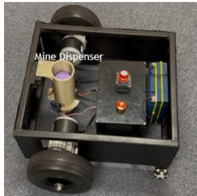
Figure 2(b): Actual prototype with mine dispenser
