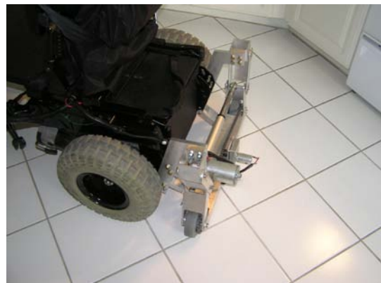
Figure 7. Sideways Wheelchair Kit (Prototype)
