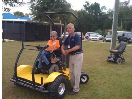
Figure 5. Beach and Rough Terrain Wheelchair Platform (Commercial Version)
