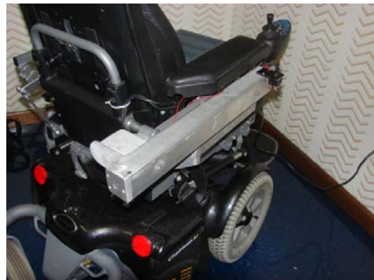
Figure 2. Backpack or Briefcase Mechanism on Powered Wheelchair (Commercial Version)
