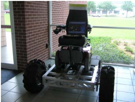
Figure 4. Beach and Rough Terrain Wheelchair Platform (Original Prototype)
